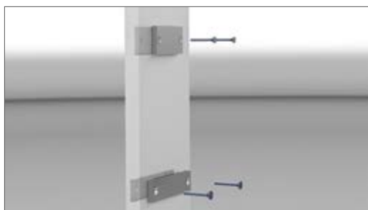
Fix base plate at the basic substructure
