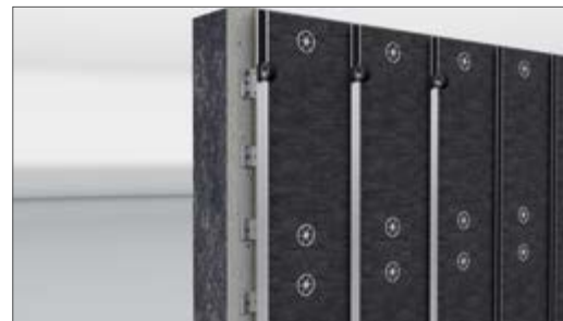
Apply joint tape on vertical bearing profiles
